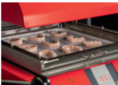
9 blanks in one thermoforming process: Biolon for Vacfomat V9
