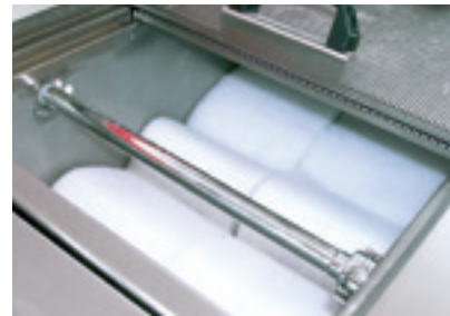
The use of filter mats saves cleaning time
